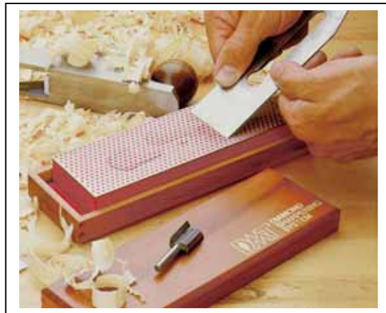
This picture shows how to sharpen a plane blade bevel on an 8" DMT Diamond Whetstone™
